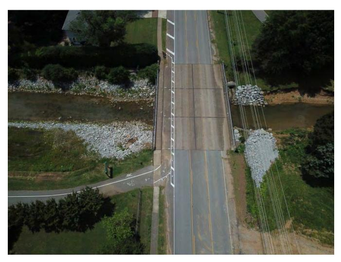
The team from Huntsville adapted their design after facing resistance to their project. Instead of shifting traffic into the under-utilized left-turn lane, they used temporary paint to create a buffered space in the shoulder for bicyclists to ride from the Aldridge Creek Greenway to the crosswalk.
